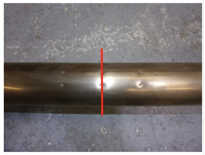
To make it easier to cut the exhaust we reccomend removing it from the car. Find the 3 pairs of indents and use the middle pair to mark out the cutting line. Cut along the line and de-bur the edges. Re-fit the original GPF and fit the Scorpion GPF-back following the line diagram above. NOTE: If fitting at the same time as our GPF delete you won't need to cut the system.
